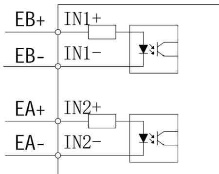
2、 External Pulses and Direction Differential Signals:
