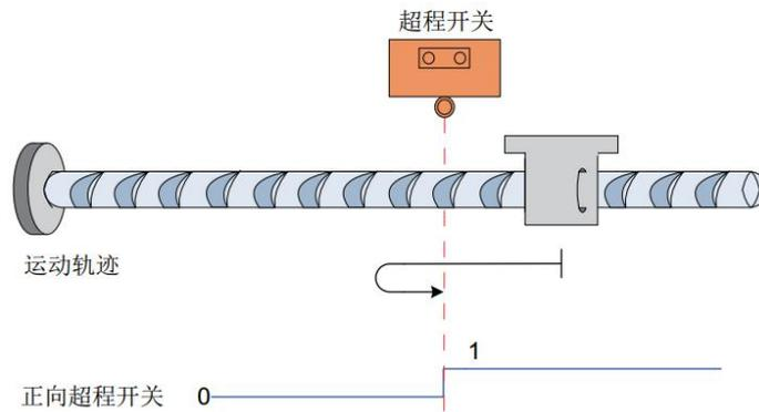
(3) Origin Zero: Forward zero, deceleration point, origin is positive limit switch(P288 x4)
