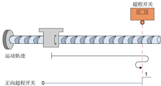
② The forward limit switch signal is valid when the motor starts to move. The motor directly reverses the forward limit switch signal to the -P290 setting point, and immediately stops after encountering the downward edge of the forward limit switch signal, then searches for the forward limit switch signal ascent slings at the P290 setting point, and in the process of positive acceleration or forward uniform operation, the forward limit switch signal is immediately stopped.
