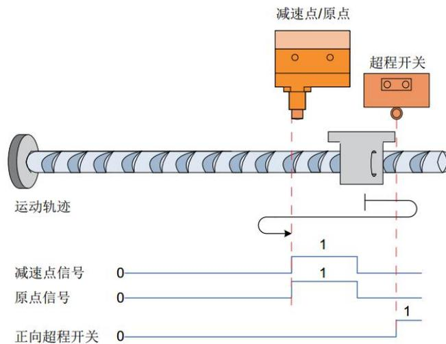
(2) Origin Zero: Forward zero, deceleration point, origin is positive limit switch(P288 x 2)
