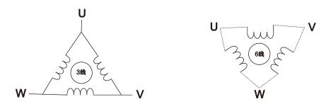
The stepping motor that the 3R60 driver can match is a three-phase hybrid stepping motor with low resistance and low inductance.
