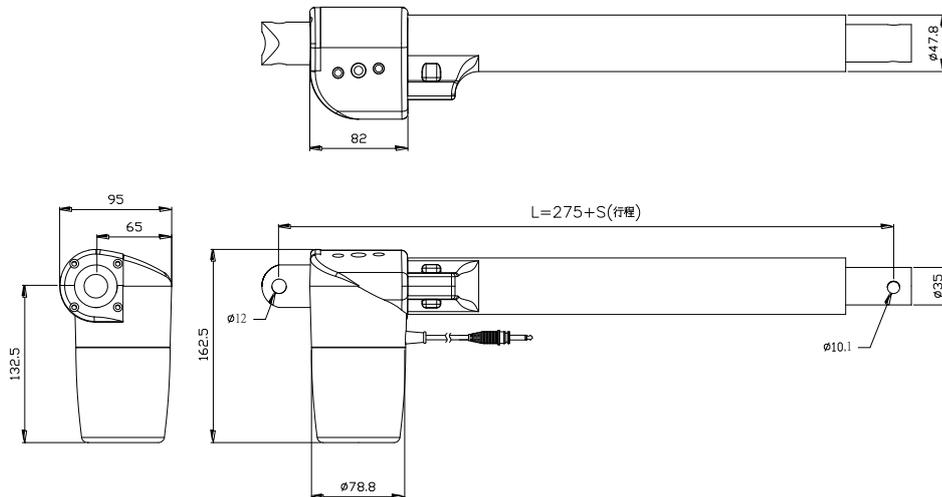
※Since August, 2012, the diameter of outer tube is 43 mm, the diameter of inner tube is 30 mm. The overload value of the control box is 6 A.
