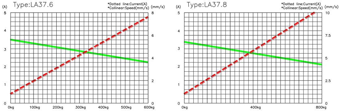
※The data above is with DC 24 V power supply. For need of data with compatible LINKAN A/C control box, please contact LINKAN A/C R&D department.
