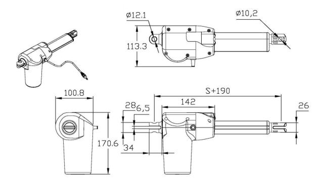
Installation Dimension for quick release (Q) function
