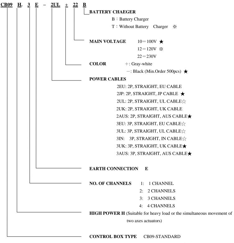
(Actuator sockets on CB09 are for Din Plug)
